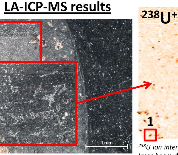
$^{238}$ U ion intensity, ablated area: 2 mm x 2 mm, 15  $\mu$ m laser beam diameter, 10 Hz laser repetition rate, 0.70 J/cm² energy density, 15 μm lateral scanning speed.
