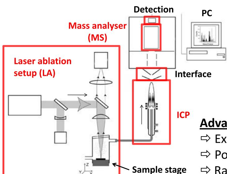
laser ablation unit or a GeoLas 200M 193 nm ArF\* ablation unit coupled to an ELEMENT XR SF-ICP-MS instrument was applied.
