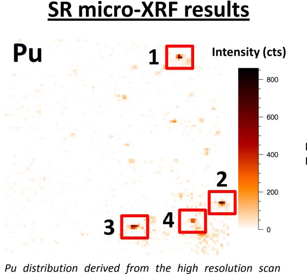
performed on case 0407. FWHM of the beam ≈ 17.5 μm, 5 s RT, image dimensions: 101 (10  $\mu$ m) x 105 (10  $\mu$ m). Plutonium map at the position of hot spot 4. FWHM beam  $\approx$  17.5  $\mu$ m, 10 s RT, 5  $\mu$ m step size.
