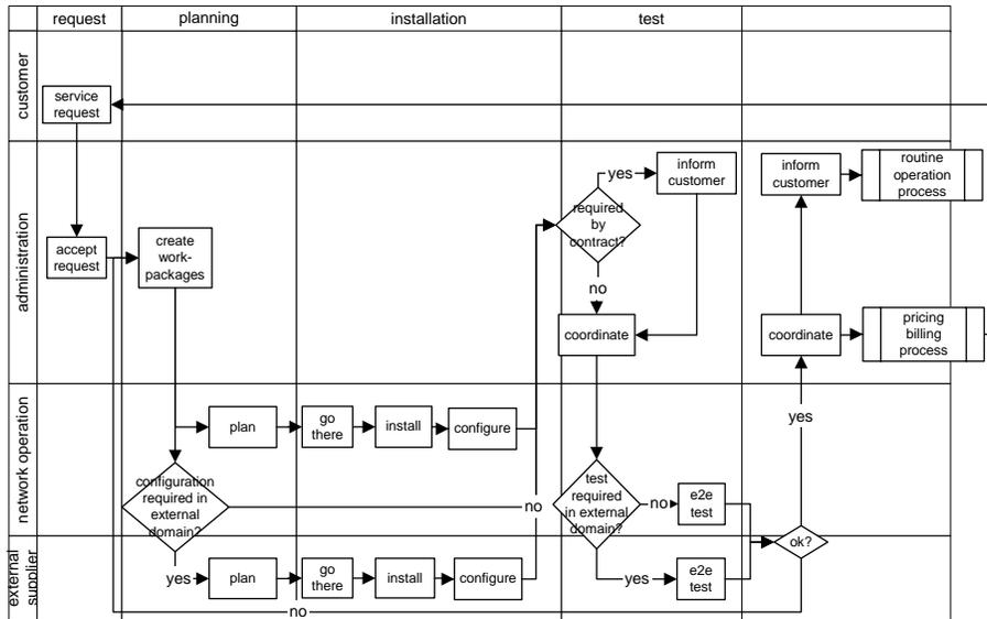
Fig. 3. Activity-based description of service provisioning process.
