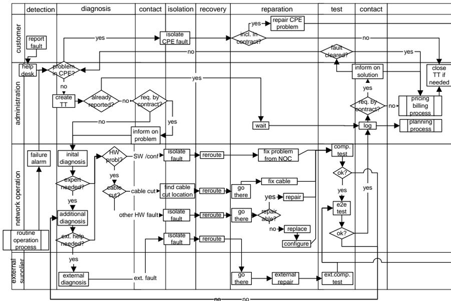
Fig. 2. Activity-based description of repair process.
