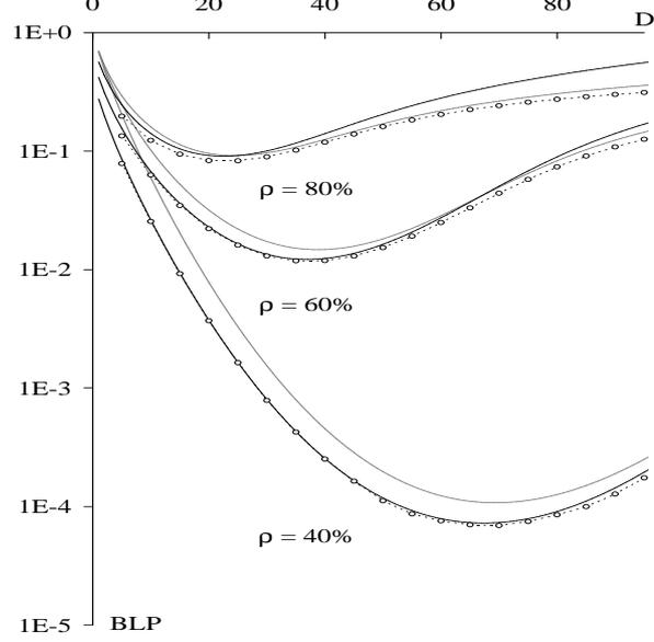
Fig. 2. BLP for exponentially distributed burst sizes ( $N = 20$ ).
