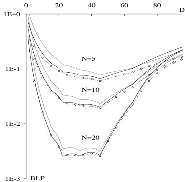
Fig. 5. BLP for a mixture of deterministic burst sizes ( $\rho = 60\%$ ).
