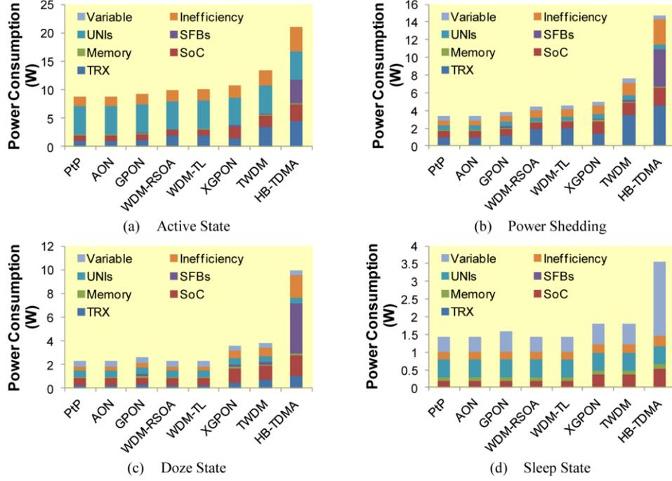
Fig. 3. Power Consumption of NGOA architectures in low power modes
