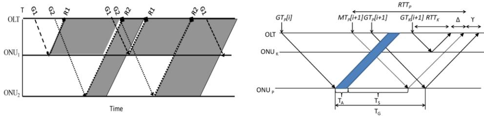
Fig. 2. (a) A TDMA-PON with an OLT and two ONUs showing REPORT (R1 and R2 for ONU1 and 2) and GATE (G1 and G2 for ONU1 and 2) messages transmission. (b) GATE prediction in the SMA algorithm.
