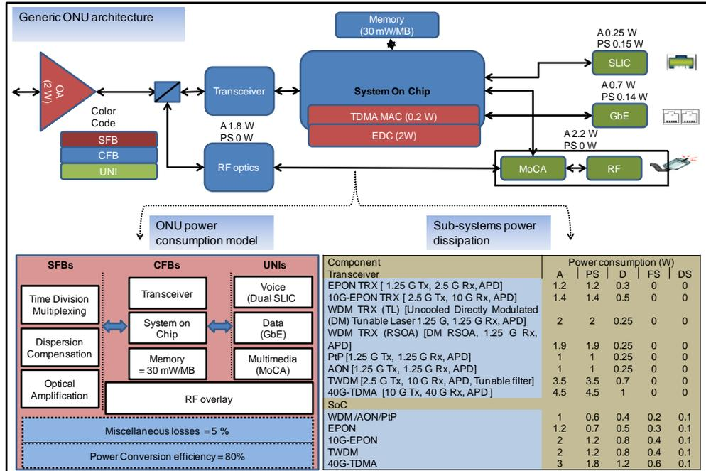
Fig. 1. ONU power consumption model.
