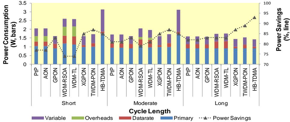
Fig. 5. Power Consumption (W) of various NGOA systems in sleep mode during busy hours with three values of the cycle length: short (5 ms), moderate (20 ms) and long (100 ms). The bars representing variable, overheads, and data rate components will be zero for the best case scenario.
