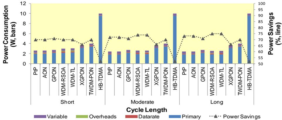
Fig. 4. Power Consumption (W) of various NGOA systems in doze mode during busy hours with three values of the cycle length: short (5 ms), moderate (20 ms) and long (100 ms). The bars representing variable, overheads, and data rate components will be zero for the best case scenario.
