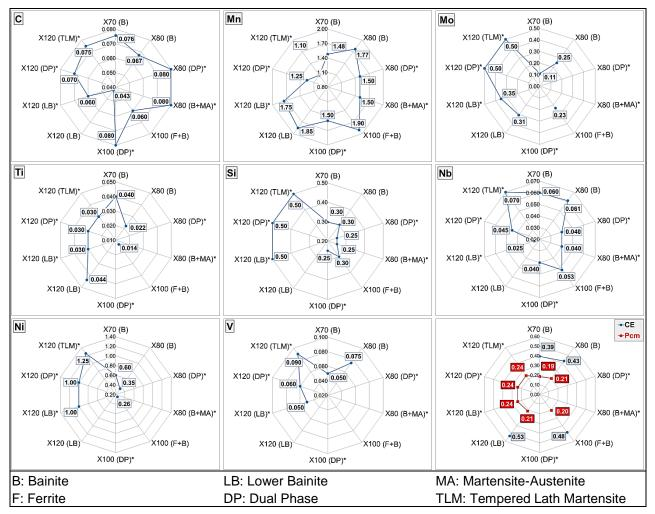
Figure 3. Overview of chemical compositions of 'conventional' and 'developed' API 5L steel grades and weldability parameters (CE and Pcm). Average results in %. Note: X120 (LB) = 0.0010 wt% B; X120 (LB/DP/TLM) = 0.25 wt% Cr.
