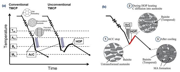
Figure 5. Schematic illustration of (a) TMCP diagram for 'conventional' vs. 'unconventional' processing and (b) microstructural changes promoted by HOP process [32].
