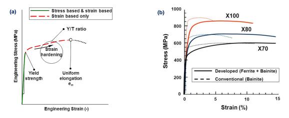
Figure 2. Relevant stress-strain parameters and stress-strain curves of 'developed' line pipe steels and 'conventional' ones (longitudinal direction) [1, 9].
