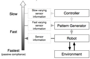
Corresponding to the biological central pattern generator we use a recurrent neural network based pattern generator of which only the output weights are trained (according to the Reservoir Computing philosophy). Such pattern generator is shown in the following illustration:
