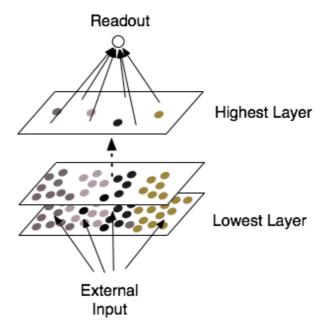
The internal reservoir weights are trained layer-wise in an unsupervised way by applying the recurrent self-organizing maps (recurrent SOMs) algorithm which is the classical SOM algorithm but generalized from the conventional static pattern domain to temporal patterns. For this, the reservoirs need to be constructed from radial basis function (RBF) units. The readout on the top layer of the hierarchy, is trained supervised by using linear regression.
