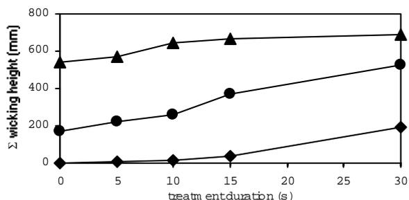
Fig. 3: Summed wicking height as function of treatment duration in an oxygen plasma. First (▲), second (●) and third (◆) wicking tests.
