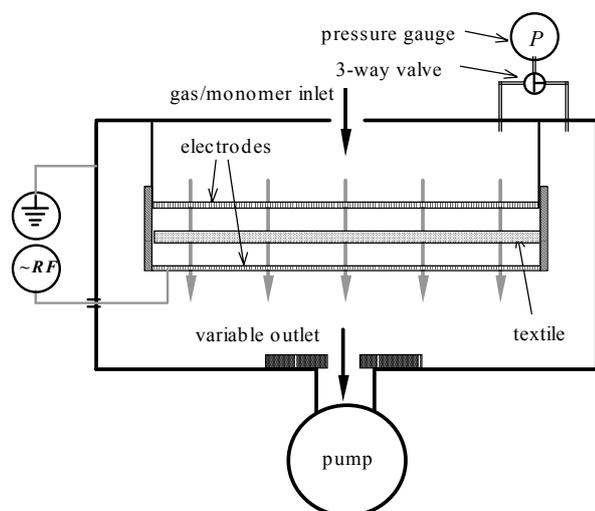
Fig. 1: Schematic view of developed reactor system
