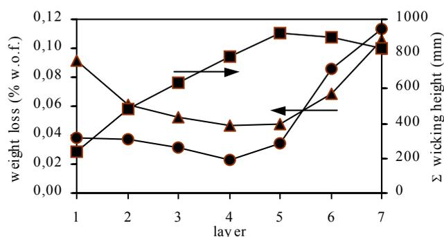
Fig. 2: Weight loss profile after a 5 minute O<sub>2</sub> plasma treatment (▲: open weave structure, ●: nonwoven). Wicking test profile after a 20 second O<sub>2</sub> plasma treatment (■: nonwoven).
