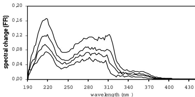
Fig. 4. UV diffuse reflectance difference spectra for plasma treated PET nonwoven (argon, 33 Pa, 28  $mW.cm^{-3}$ , 2 (top), 5, 10 and 15 min. treatment duration).
