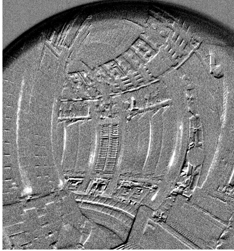
Figure 3.13: Wide angle IR camera (KL7) image of the 8 s He/D 2 (90/10) JET ICWC discharge 78579: P_{\text{RF,gen}} = 200 - 350 \text{ kW} and p = 1 \cdot 10^{-5} \text{ mbar} during the discharge. Particle transport along magnetic field lines caused heating of field line intersecting wall elements (brighter areas).
