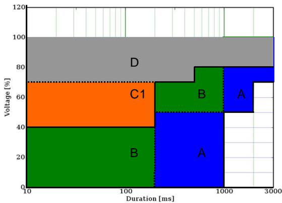
Fig. 3. Equipment Immunity Classification for unbalanced (type I and II) voltage dips
