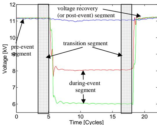
Fig. 2. An example of a typical voltage dip - rms voltage plot, with indicated event and transition segments
