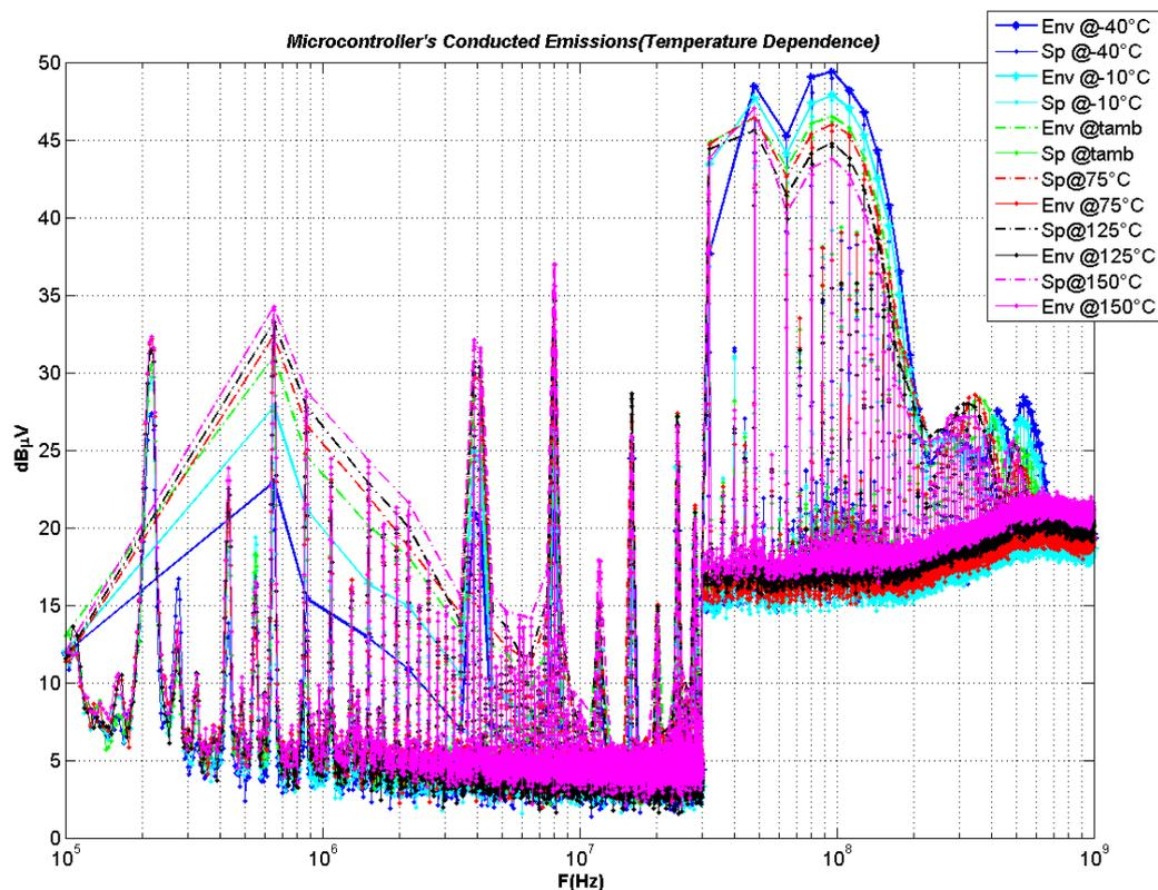
Figure 1. EMI-signature of a microcontroller at different temperatures
