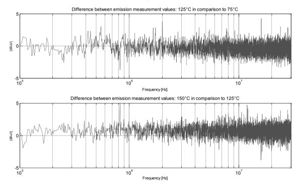
Figure 4. Difference between measurement at 125°C and 75°C (top) and 150°C and 125°C (bottom)
