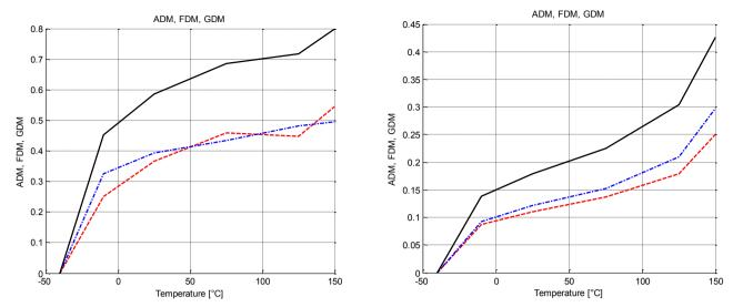
Figure 3. FSV-results (ADM red dashed, FDM blue dashed-dotted, GDM black solid) for frequency range 100 kHz – 30 MHz (left) and 30 MHz – 200 MHz (right)
