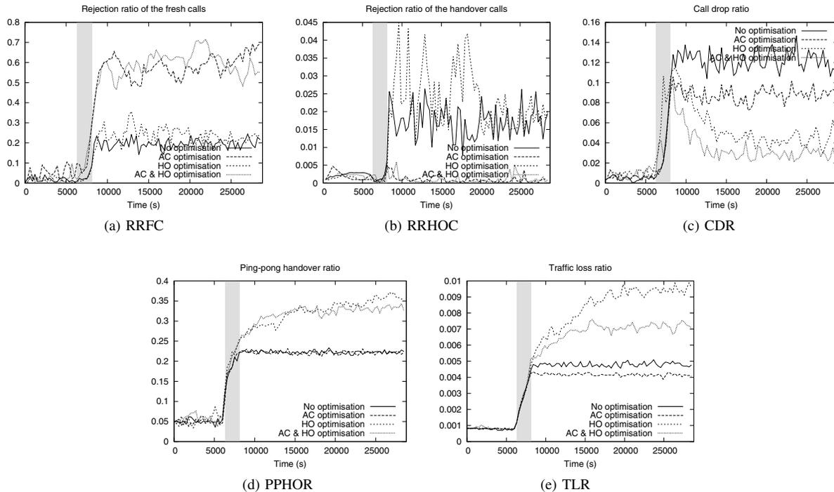
Fig. 3: The AC and HO performance metrics of scenario 5, plotted over time.
