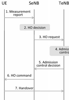
Fig. 1: A sequence diagram showing the steps of the HO procedure.
