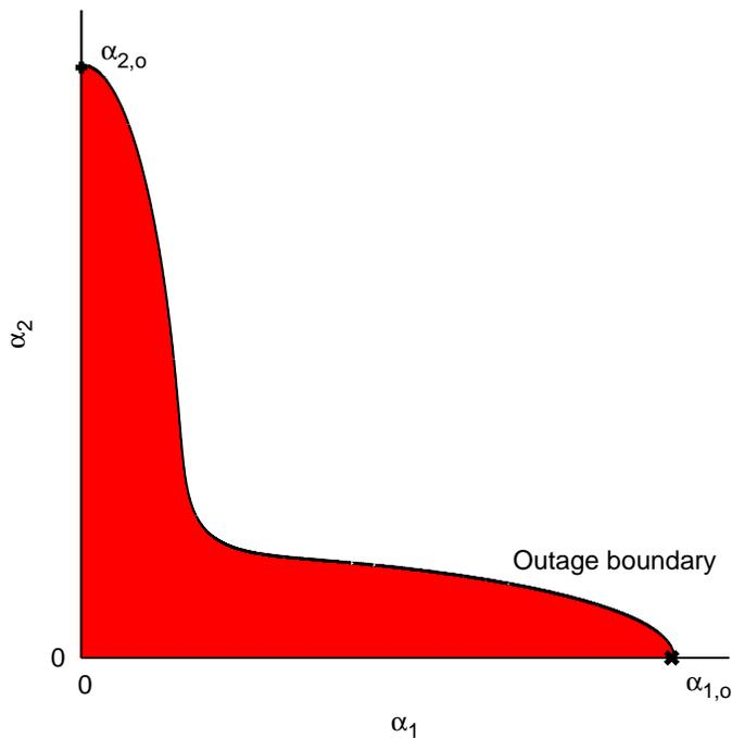
Figure 2: The outage boundary limits the region  $V_o$  (coloured red) in the fading space which corresponds to an information theoretic outage event. The points  $\{\alpha_{b,o}, b = 1, \dots, B\}$  are shown for  $B = 2$ . The information rate is  $R = 0.9$  bpcu. The average SNR is fixed to  $\gamma = 8$ dB.
