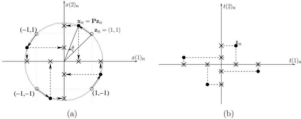
Figure 1: Displaying the rotation at the transmitter (a) ( $\mathbf{x}_n$ ) and at the receiver (without noise) (b) ( $\mathbf{t}_n$ ) for  $B = 2$ . The empty (filled) circles represent  $\Omega_z$  ( $\Omega_x$ ). The components of  $\mathbf{t}_n$  are obtained by scaling the components  $\mathbf{x}_n$  by their respective fading gain (here  $\alpha_2 < \alpha_1$ ). The crosses on the coordinate axes are the transmitted and received vector components, respectively.
