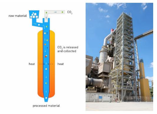
**Figure 1.** Left: shematic section of the LEILAC1 capture plant. Right: LEILAC1 capture plant at the Lixhe cement factory.
