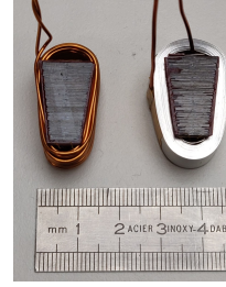
Fig. 4. Prototype tooth coils. Left: enamelled copper wire tooth coil, Right: anodised aluminium foil tooth coil
