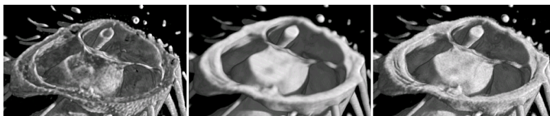
Fig. 4. Horizontal cut through the 3D rendered model of the reconstructed leg. Left: FBP, middle: MBA, right: BAC.
